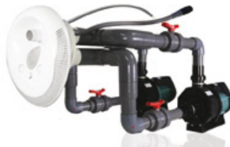
Emaux Counter Current Jet system has a flow-rate of up to 90m³ per hour. All controls can be operated from inside the pool so you don't have to get out of the water to adjust the settings. The adjustable nozzle allows a better control of the water flow while the underwater bubble switch can control the bubble effect of the flow.
